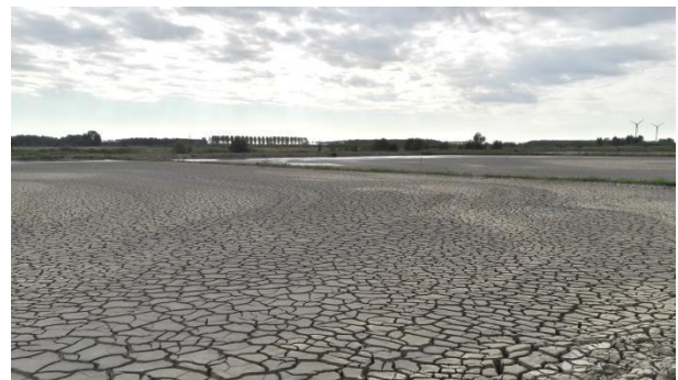
Figure 3. Image of one cell of the Kleirijperij taken on 16th of August (day 135), therefore about one month after the second layer was deposited. Photo EcoShape.
