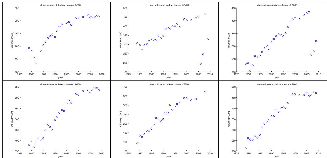
Figure A 2. Examples of dune volumes at Schiermonnikoog, at the location where new dune development from around 2000 on resulted in a green beach. NB: the landward reference varies between transects. Therefore only trends can be compared and not absolute volumes.
