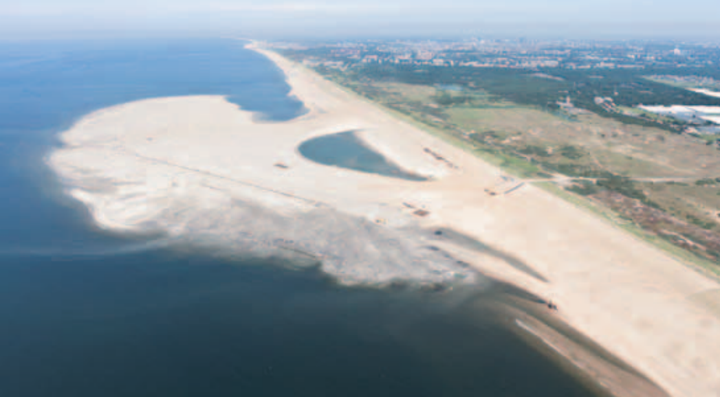
Figure 5. Delfland Sand Engine on June 14, 2011 showing the progress of construction of the peninsula which will extend about 1 km into the North Sea.
