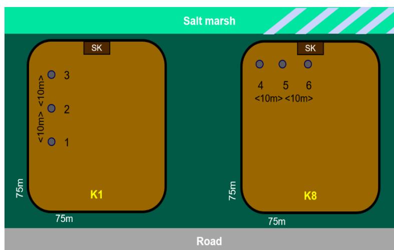
Figure 2.4 Schematic overview (not scaled) showing placement of the respiration chambers in plot K1 and K8. SK = Dewatering cistern.
