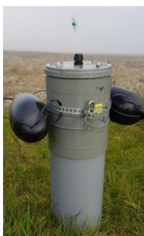
Figure 2.3 Cylindrical respiration chamber for sampling greenhouse gases in the field.
