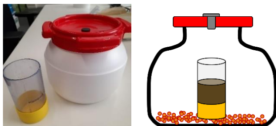
Figure 2.5 Closed vessel with sample of dredged material to measure GHG emissions semi-continuously under controlled conditions.
