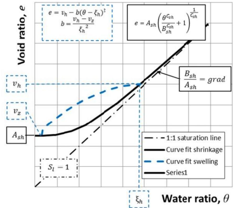
Figure 1 – Shrinkage curves
